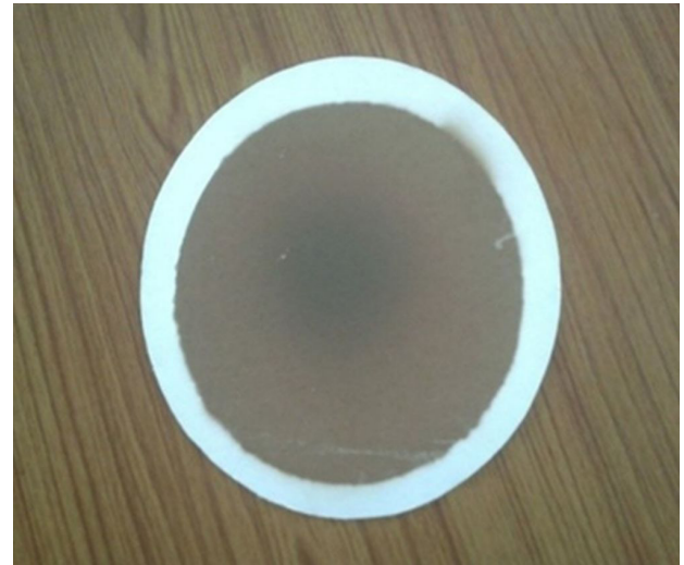
Fig. 3. Filter paper with extracted fumes using CO 2
