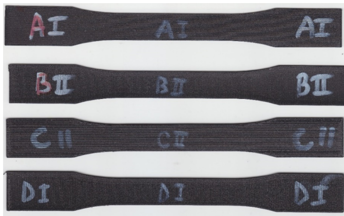
Fig. 3. Printed specimens divided into series according to adjusted printing parameters
