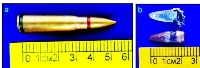
Fig. 5. Photographs of \text{Ø}7.62 \times 51 mm HSC projectile (a) before impact (b) recovered projectile after penetration
