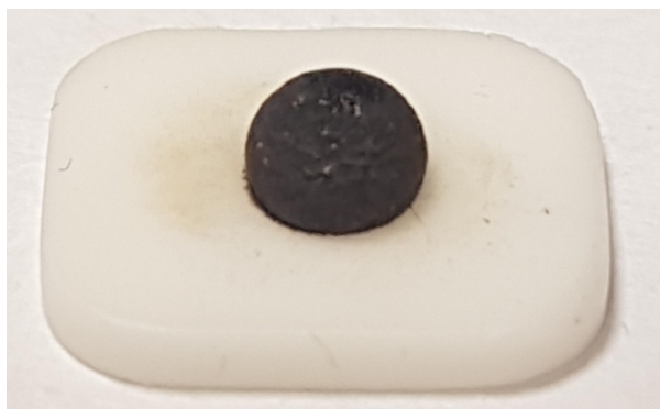
Fig. 2. Melted sample of CuSn10 tin bronze inside high temperature microscope
