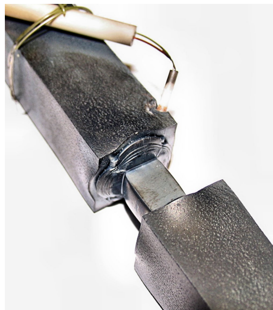
Fig. 4. Detail of thermocouple, deformation zone and adjacent areas of the sample after forming by alternating compressions
