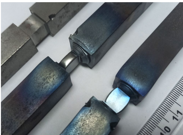
Fig. 9. Central parts of samples before deformation (above) and after simulations
