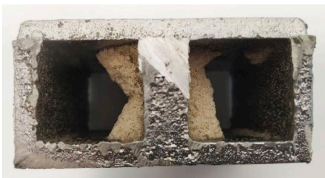
Fig. 12. Test casting after core discharge
