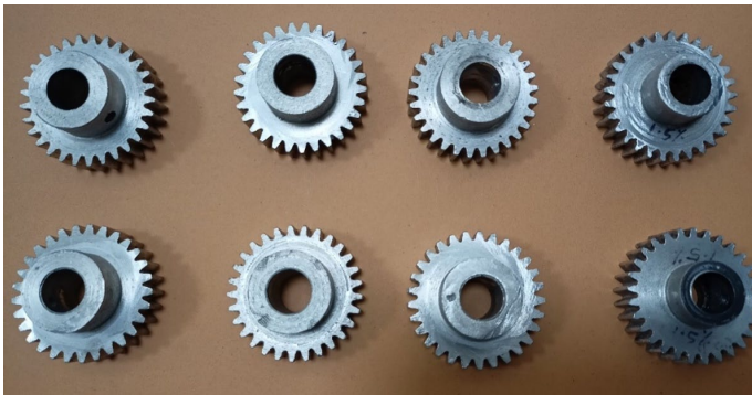
Fig. 4. Manufactured Al-nano \text{Al}_2\text{O}_3 composite spur gears
