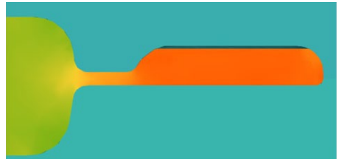
Fig. 8. Failure to fill the discharge groove in the absence of lubrication
