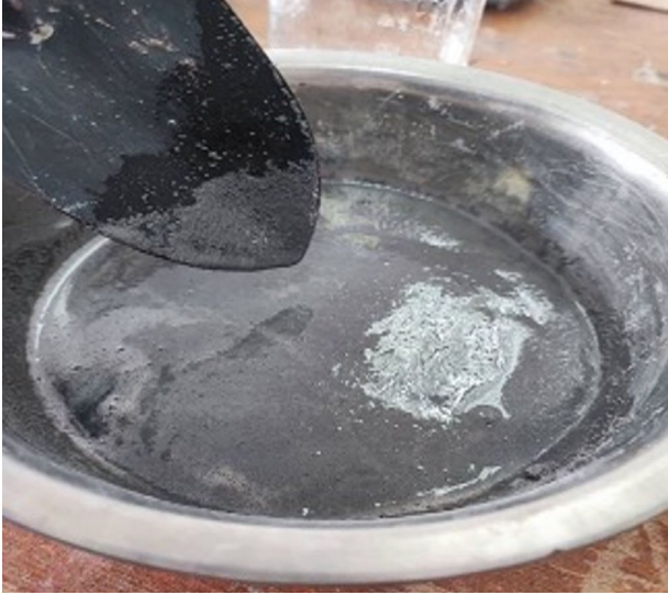
Fig. 7. The coating mixture of silica fume based geopolymer at 1.0 S/L ratio
