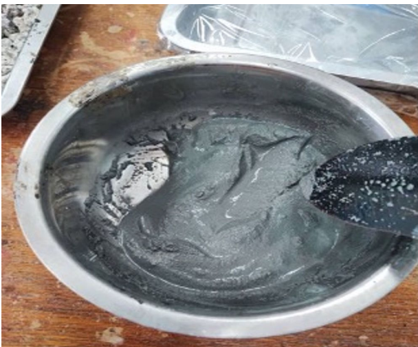
Fig. 8. The coating mixture of silica fume based geopolymer at 1.8 S/L ratio
