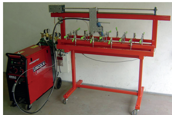
Fig. 1. Apparatus for welding with micro-jet cooling
