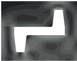
Figure 19. Effective stress distribution in the mold after 60 s (case B). Maximum value (191 MPa) is marked in light gray, while minimum value (95 Pa) is marked in black
