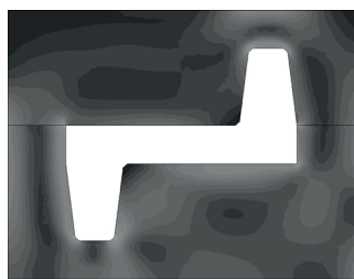
Fig. 12. Effective stress distribution in the mold after 60 s (case A). Maximum value (217 MPa) is marked in light gray, while minimum value (350 Pa) is marked in black
