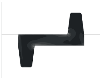
Fig. 11. Effective stress distribution in the casting after 60 s (case A). Maximum value (0.27 MPa) is marked in light gray, while minimum value (350 Pa) is marked in black
