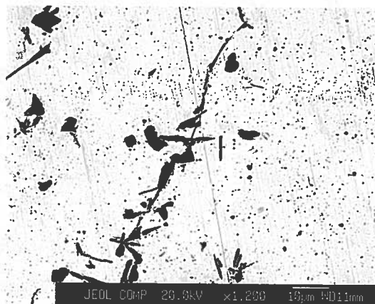
Fig. 3. Micrograph of specimen No 5, "as cast". The photo has been taken in secondary electrons. The black crystals are of Ti_5Si_3 and Ti_5Si_4 . The light matrix is tin rich. The composition of the tiny crystals could not be measured
