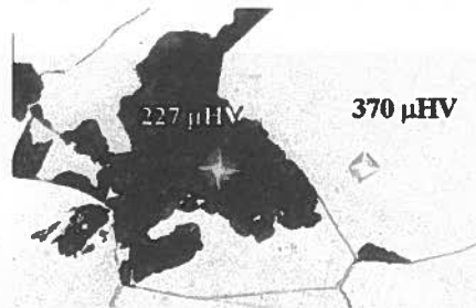
Fig. 7. Microhardness of cellular precipitates and the grains inside in CuNi13Sn5 alloy aged at 400°C for 7 \times 10^2 minutes
