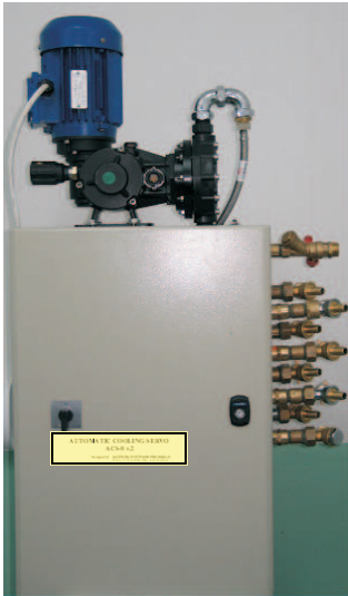
Fig. 1. Automatic Cooling Servo device
