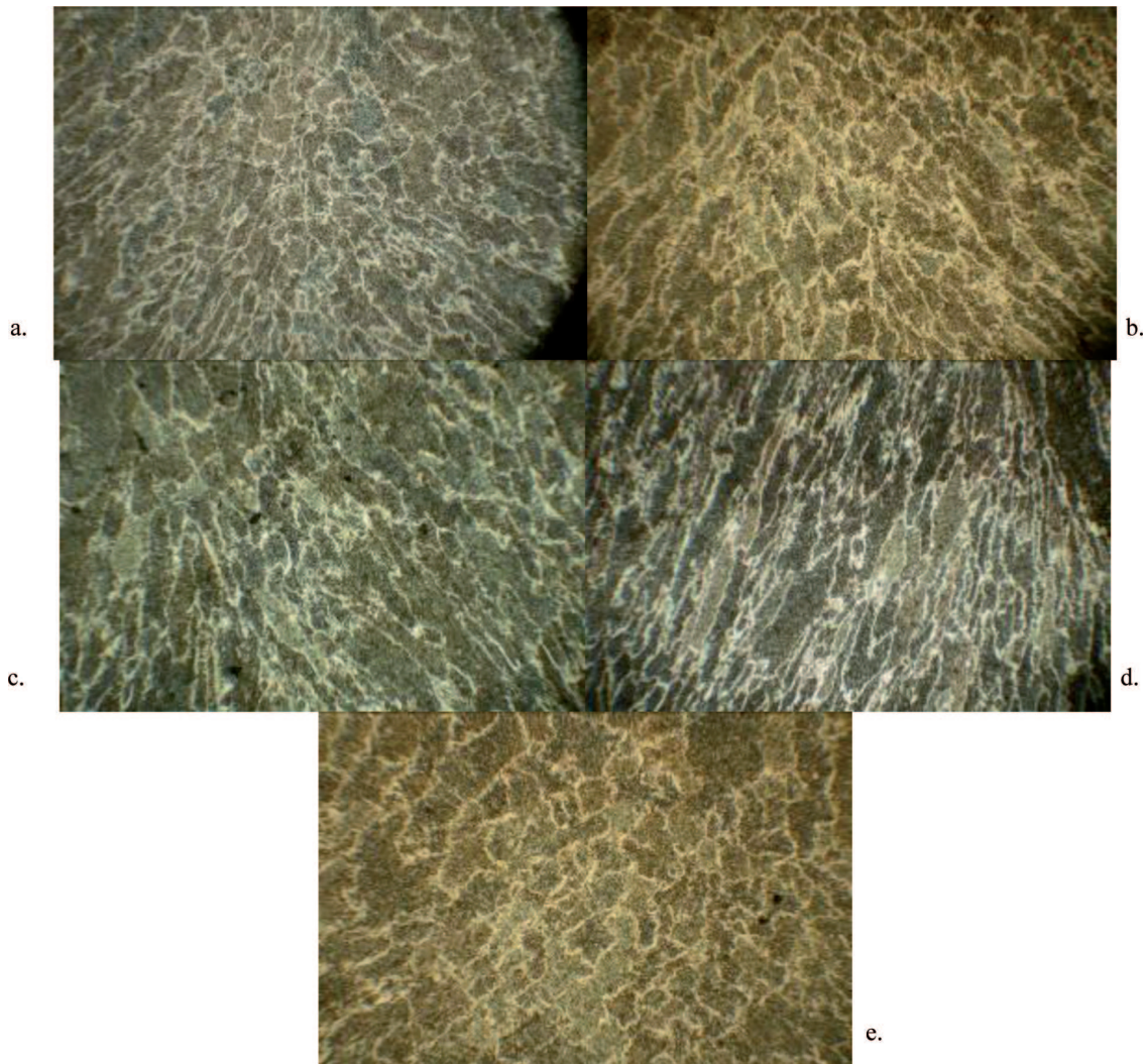
Fig. 6. Example of typical analyzed structures for MIG: a) standard MIG; b) MIG with micro-jet (X 0.4); c) MIG with micro-jet (X 0.6); d) MIG with micro-jet (Y 0.4); e) MIG with micro-jet (Y 0.6). Magnification x 30
