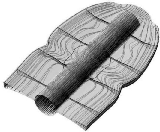
Fig. 7. 3D distribution of the grid in the model of a shaft forging (the charge diameter being 40 mm)
