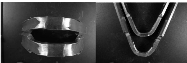
Fig. 7. Results of bend test – root side
