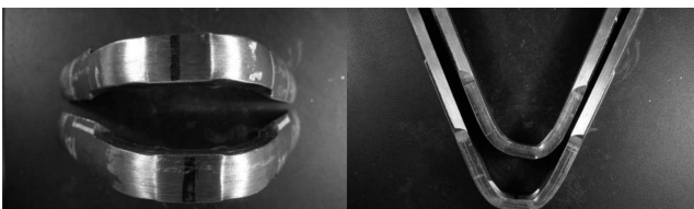
Fig. 6. Results of bend test – face of weld
