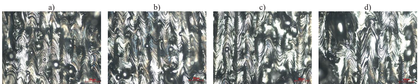
Fig. 6. Light microscope images represents the differences of SLM parts made: (a) h=25 μm, t=25 μs; (b) h=25 μm, t=100 μs; (c) h=100 μm, t=25 μs; (d) h=100 μm, t=100 μs; mag. 1000x
