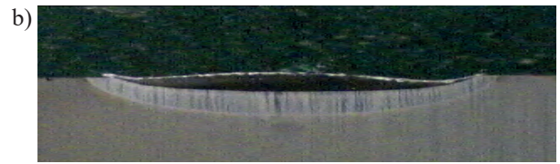
Fig. 6. The cross - section of laser surface alloyed 32CrMoV12-28 steel after laser alloying with a) WC powder and b) VC powder at laser beam power of 2.3 kW
