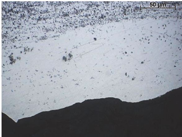
Fig. 8. Structure of the AlSiCu3 PM material anodised surface layer with 10% Al 2 O 3 powder addition
