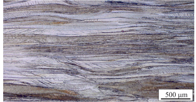
Fig. 1. Microstructure of the HE copper, \epsilon = 2.24 ; longitudinal section of the sample
