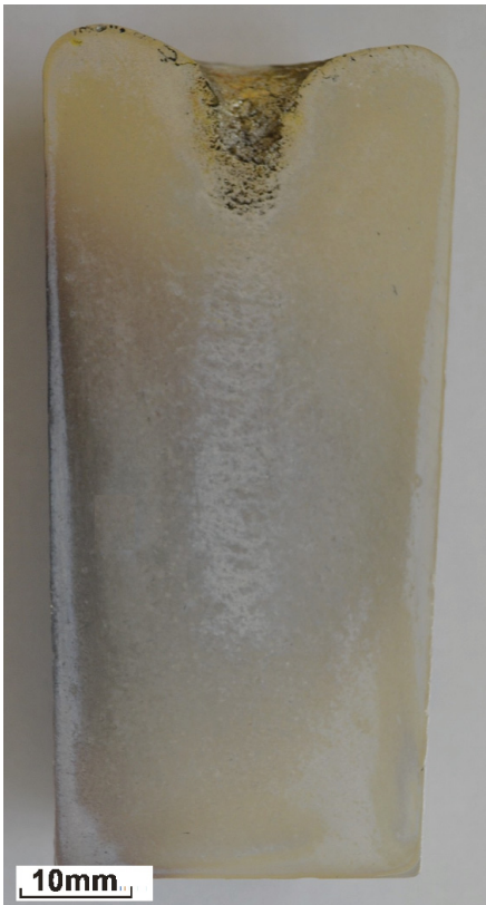
Fig. 1. Cross-section of ingot from LAZ441 alloy
