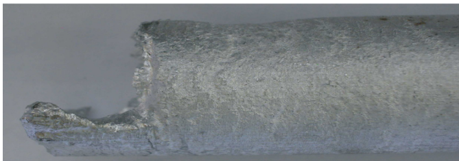
Fig. 9. View of the broken aluminum ingot in studied horizontal continuous casting process
