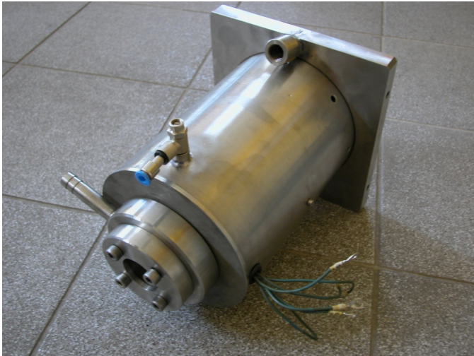
Fig. 4. View of the water cooled continuous casting mould
