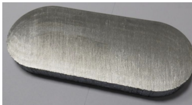
Fig. 1. The plate cut from a casting
