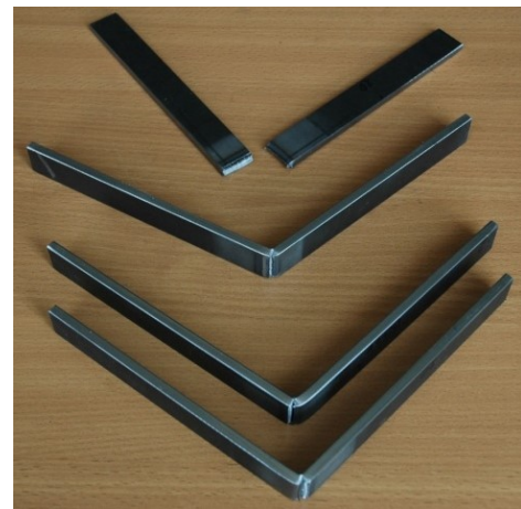
Fig. 6. A view of the samples after technological bend test of 5.0 mm thick butt joints of STRENX 1100 MC steel autogenous laser welded by the Disk laser, evaluated according to the PN-EN 895 standard (from the bottom 2 test samples of joint B and A respectively)
