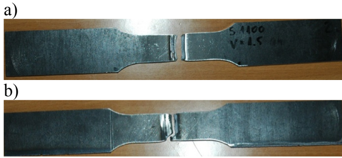
Fig. 7. A view of the broken samples from the tensile tests of butt joint A welded at 3.3 kW and welding speed of 1.5 m/min (energy input of 132 J/mm) (a) and the joint B welded at 3.3 kW and welding speed of 1.0 m/min (energy input of 198 J/mm) (b)
