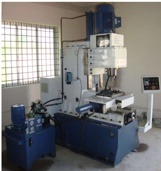
Fig. 1. Photographic View of the FSW Machine (Semi Automatic) employed in this investigation
