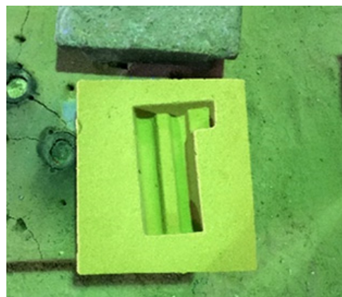
Fig. 1. Sand Casting Mould
