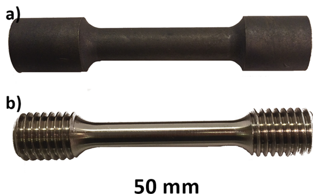
Fig. 2. Geometry of prepared element after: a) excision b) machining
