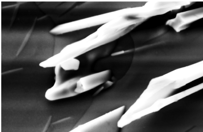
Fig. 10. Phenomenon of branching recorded in the irregular L-shape, rod-like eutectic structure; almost plane s/l interface exposed between main rod and its branch: a) structure without any correction, b) new color superposed over the frozen liquid to make the planar s/l interface well-marked
