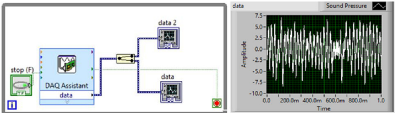
Fig. 4. Lab VIEW program for Data Acquisition
