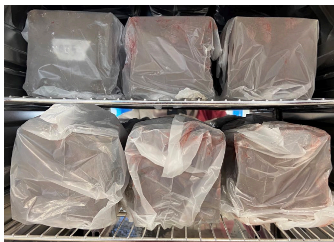
Fig. 1. Oven curing process of geopolymer concrete
