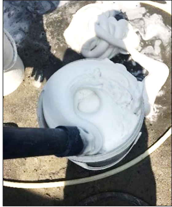
Fig. 1. The stable foam generated from the TM-1 foam generator
