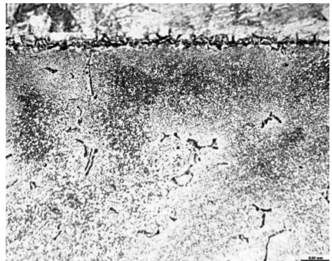
Fig. 5. Microstructure of the stainless steel (X2CrNi 18-9) joint brazed with BAG-19 alloy. Upper part – stainless steel, lower part – braze
