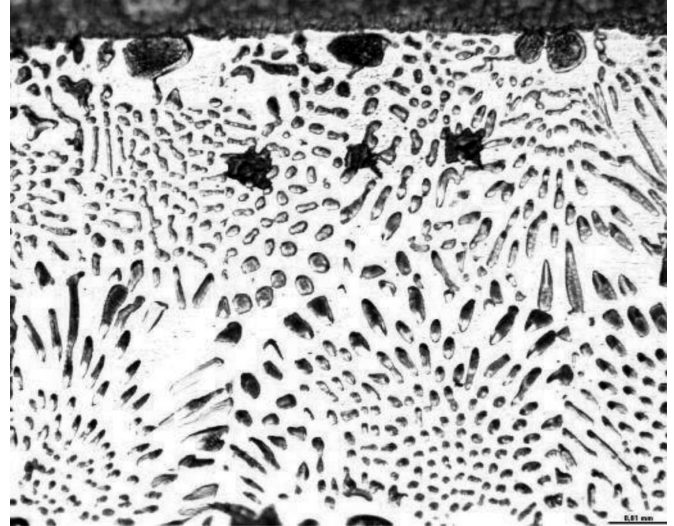
Fig. 4. Microstructure of the stainless steel (X2CrNi 18-9) joint brazed with BAG-8a brazing alloy. Upper part – stainless steel, lower part – braze
