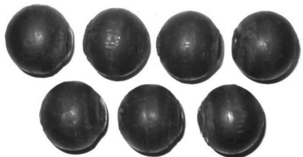
Fig. 7. Balls formed in the rolling process in multiple helical impressions
