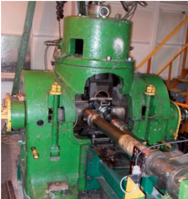
Fig. 5. Skew rolling mill built in the system of two triple helical rolls, in which rolling tests of balls S030 mm were conducted
