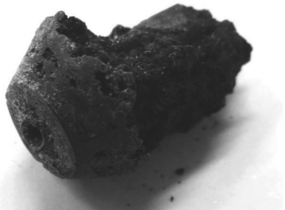
Fig. 8. Sintered lubricant removed from the exit bell of a die after drawing process at a speed of v = 25 m/s
