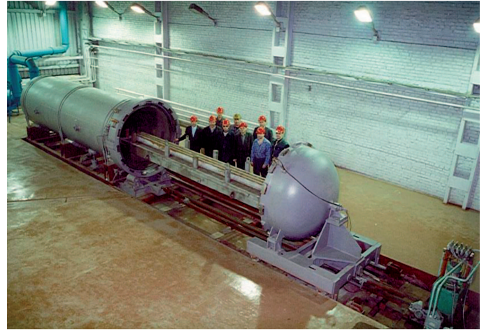
Fig. 6. Explosion Chamber KVG-8
