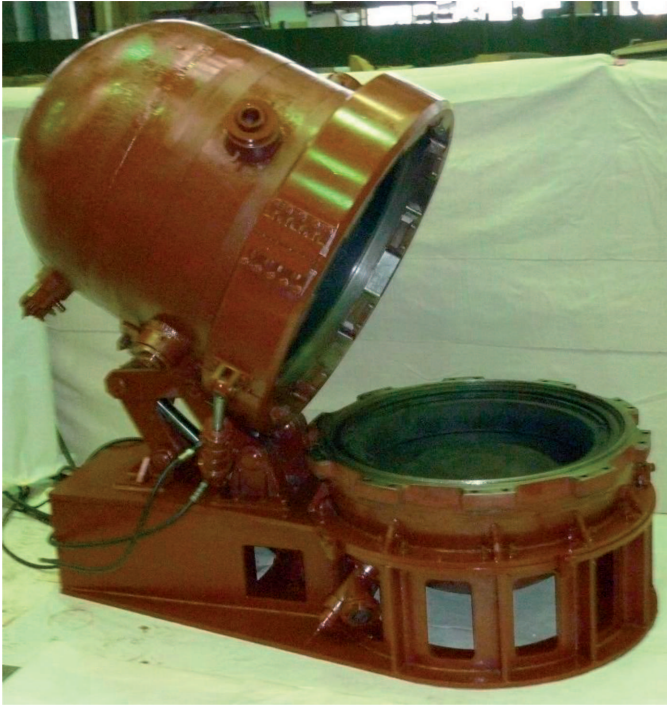
Fig. 4. Explosion Chamber KV-2
