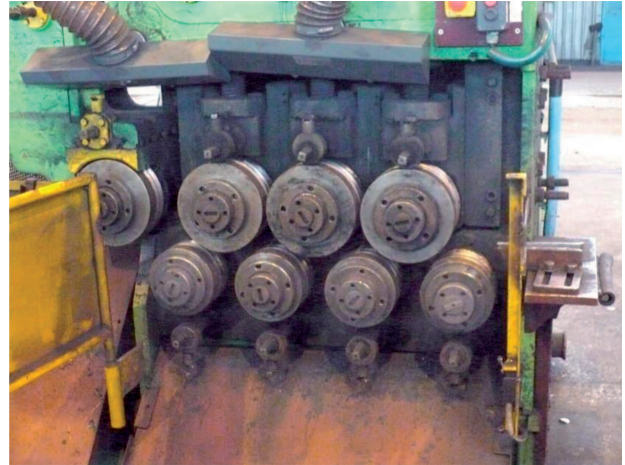
Fig. 1. Photograph of the roller straightener used for the controlled cold working deformation of rods of the S235JR steel
