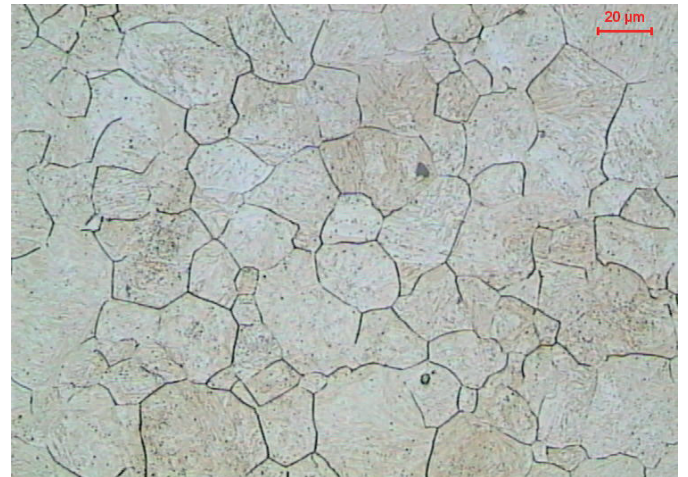
Fig.2. Typical microstructure of the prior austenite in a structural steel
