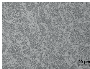
Fig. 10. Microstructure of S460 steel, ferrite + bainite + martensite ( v_H = 2600 K/s i v_{8/5} = 20 K/s)
