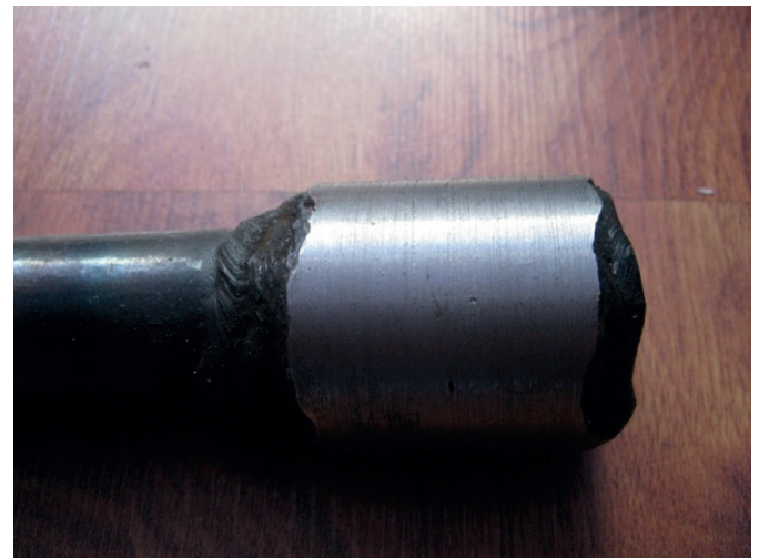
Fig. 2. The superficial deposit made by using welding with micro-jet cooling [21]
