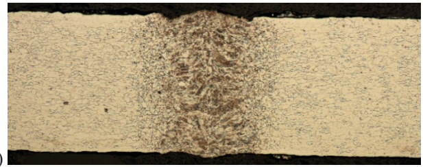
Fig. 6. Cross sections of the bead-on-plate welds produced on the 0.8 mm thick electro-galvanized steel sheet DC04 by a disk laser at very similar heat input, Table 3; a) bead B4 (750 W, 2.0 m/min, 22.5 J/mm), b) bead B8 (2000 W, 6.0 m/min, 20 J/mm)
