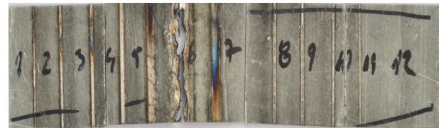
Fig. 3. A view of the bead-on-plate welds produced on the 0.8 mm thick electro-galvanized steel sheet DC04 by a disk laser, Table 3
