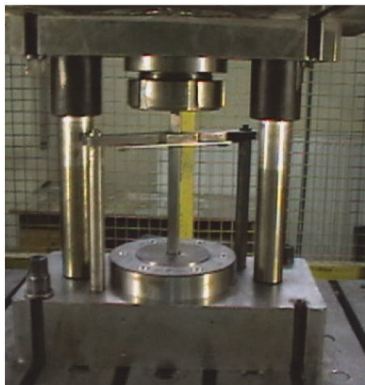
Fig. 8 View of the tool for backward extrusion, MESKO S.A. company
