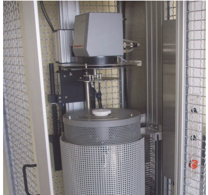
Fig. 2. Photograph of rotational viscometer used in investigations The chemical composition of investigated Stellite™ 21 alloy is shown in Table 1.
