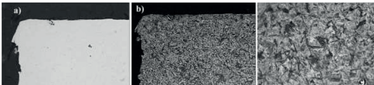
Fig. 4. Results of metallographic analysis for the stabilizer bar subjected to shot peening (Source TKF & s)
