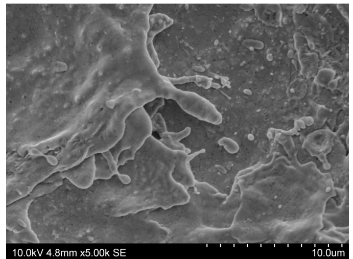
Fig. 6. Drops of metal on the contact surface resulting from local partial melting by electric arc. Sample after 250 thousand cycles
