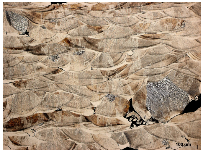
Fig. 2. Microstructure of SLM stainless steel type AISI 316L
