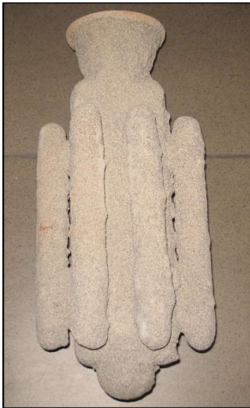
Fig. 1. Ceramic mould for strength test of castings
