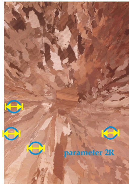
Fig. 3c. Approximate method of the R_{exp} – tip radius measurement within the columnar structure surrounding the single crystal situated axially in the brass ingot
