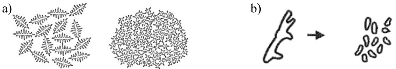
Fig. 3. Schematically model of effect of technological processes on structural features in aluminium alloys [37,38]; (a) refiners effect onto Al-matrix; (b) modifiers effect onto eutectic Si particles
