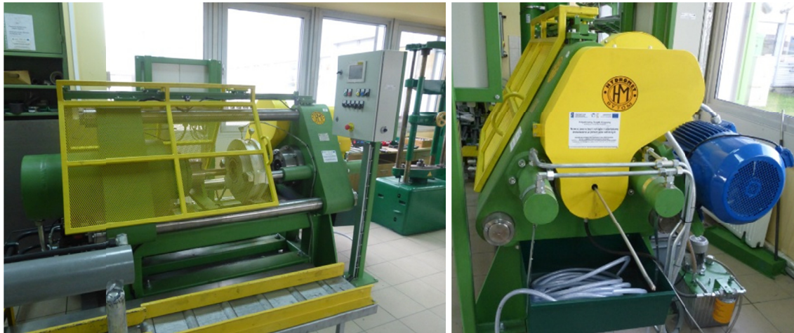
Fig. 4. Hydromet hydraulic KoBo 2,5 MN press used in the experiment
