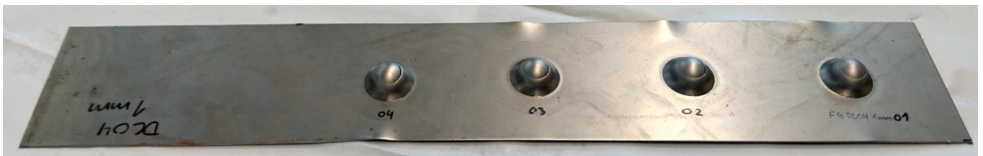
Fig. 7. DC04 steel sheet specimen of 1 mm in thickness used for the Erichsen test
